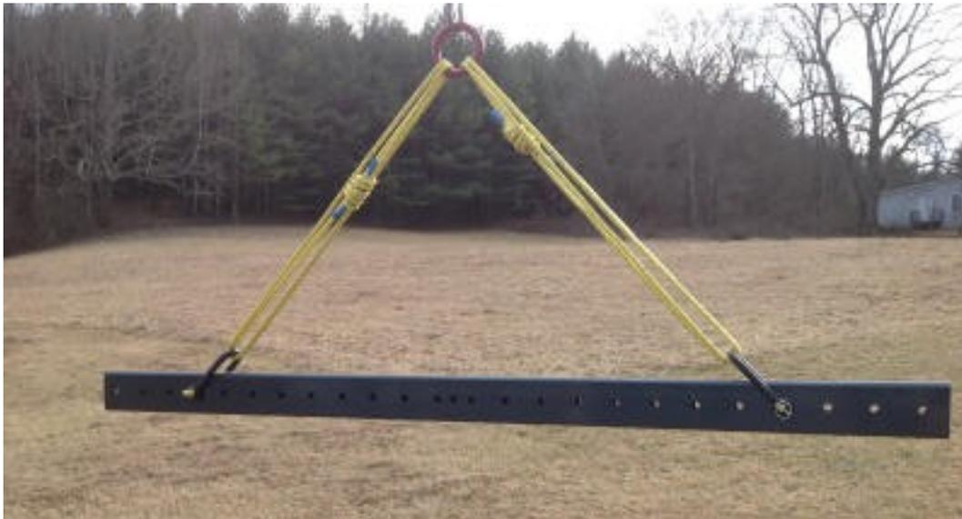
The lower parts of the bar can be configured either as a “standard” bar, or as an “instant release bar”. The standard bar uses simple shackles, while the instant release incorporates ram hooks that can be activated from a distance to remotely release any slings or load below.
